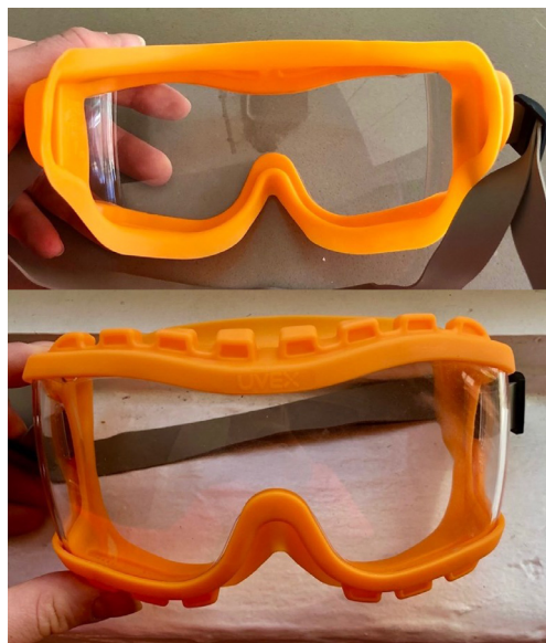
Figure 1—Protective eyewear. The patient used these goggles, shown from the back (top) and front (bottom), and cleaned them after each patient encounter with Super Sani-Cloth® Germicidal Disposable Wipes (PDI Healthcare). The goggles provided a tight seal over the upper brow where the original site of discharge occurred.
